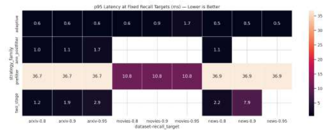
Figure 6. p95 latency for a fixed Recall@20 target.
