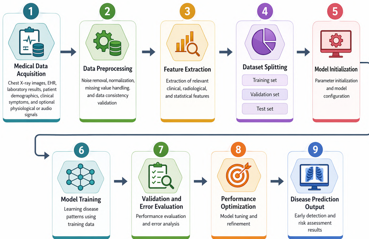
Figure 1. Workflow of the proposed AI-driven healthcare software system for early detection of chronic mycobacterial lung disease.
