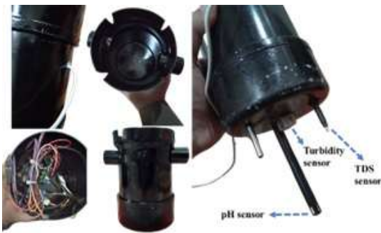
Figure 2. Exterior casing and sensors.
