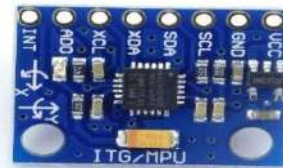
Figure 4 MPU6050 Accelerometer to calculate the angular velocity and acceleration of wheelchair.
