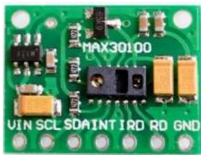
Figure 2 MAX30100 Heart Rate Oxygen Pulse Sensor for determining heartbeat along with oxygen saturation.
