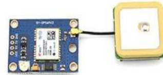
Figure 7 NEO-6MV2 GPS Module to determine the geographic location of the user.
