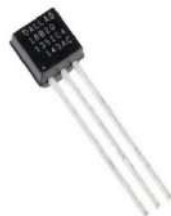
Figure 3 DS18B20 Digital Sensor used for determining temperature.
