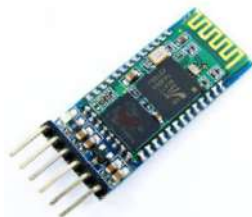
Figure 11: HC-05 Bluetooth Module for connecting mobile app with the system.
