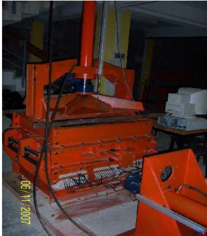
Figure 3.1 The Pullout Test Device
